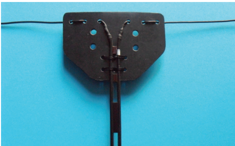
PHOTO 1: The feed point centre used for the OCFD antenna (the white mark denotes the longer wire leg's connection).
