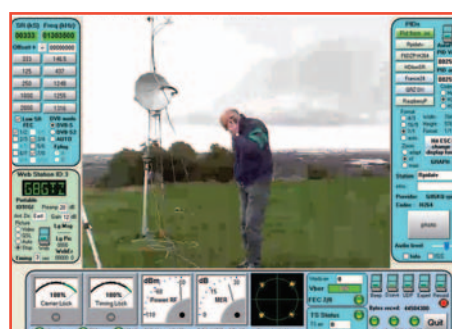
FIGURE 3: G8GKQ/P using a Portsdown Tx on 146MHz over a 60km path, received via MiniTiouner.
