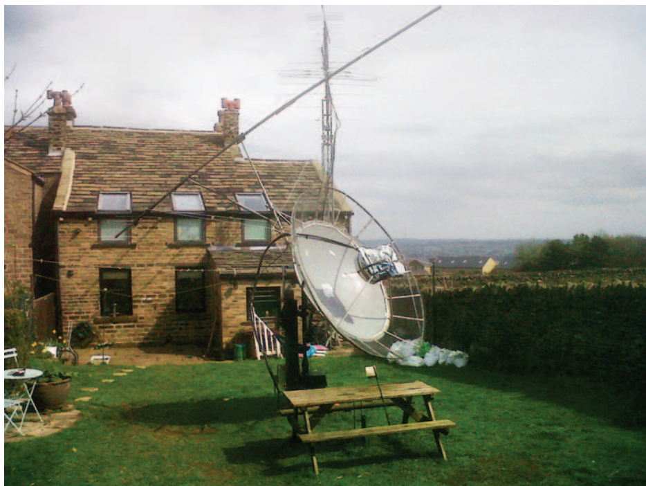
PHOTO 1: A small 23cm EME installation as described in the text. Note the 2m Yagi above the dish.
