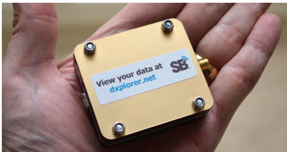
The tiny WSPRlite transmitter.
